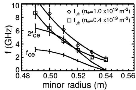
FIG. 6. Edge profiles for cyclotron and upper hybrid frequencies for  $\bar{n}_e = 0.4 \times 10^{19} \text{ m}^{-3}$  and  $1.0 \times 10^{19} \text{ m}^{-3}$ . These frequencies include the port-hole perturbation to the equilibrium magnetic field, unlike Fig. 1.
