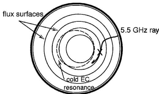
FIG. 2. Poloidal flux and a constant  $|B|$  (resonance for 5.5 GHz) surface. The 2D equilibrium is a solution of the Grad-Shafranov equation fit to the available magnetic data. The position along the ray where the optical thickness is 1 is labeled (x) to indicate the location of the source of observed emission.
