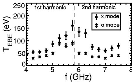
FIG. 4. Measured O- and X-mode radiation temperature vs frequency. The vertical dashed line at 5.8 GHz separates two cyclotron harmonics.
