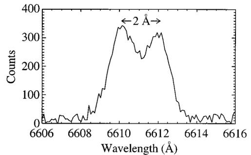
FIG. 4. Measured spectrum of Doppler shifted  $H_\alpha$  emission from beam using vertical polarizer showing Stark splitting of  $\pi^+$  and  $\pi^-$  components.
