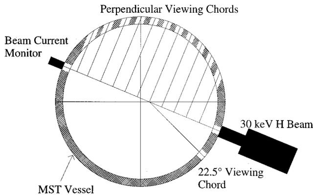
FIG. 1. Poloidal cross section of MST showing location of diagnostic neutral beam and several viewing locations.
