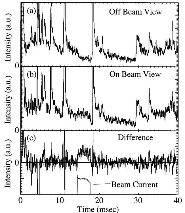
FIG. 2. Measured C VI (3433.69 Å) emission intensity for central views: (a) just to the side of and (b) intersecting the beam and (c) the difference of the two views.
