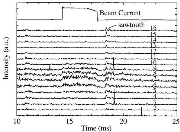
FIG. 3. Measured emission in 16 wavelength channels centered on the C VI emission at 3433.69 Å.
