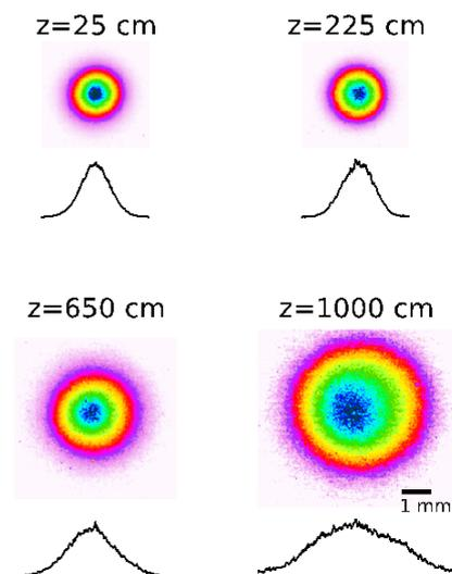
**Figure 2.** Beam intensity profiles recorded by a DataRay beam profiling camera at various distances from the laser source. The graph below each profile is a 1D cut through the center of each 2D profile.
