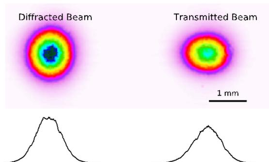
**Figure 5.** Beam intensity profiles of the diffracted (deflected) and transmitted (zero-order) beam. The graph below each profile is a 1D cut through the center of each 2D profile.
