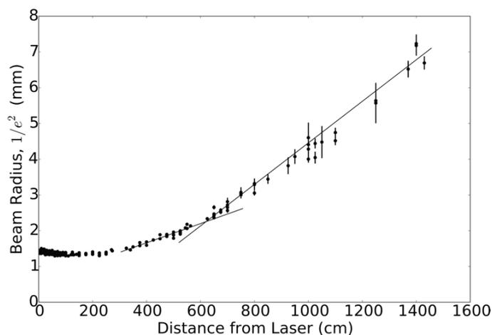
**Figure 3.** The variation of the  $1/e^2$  beam radius as a function of distance from the laser source. The two lines illustrate the mid-field divergence (300–600 cm from laser) and the far-field divergence (600–1400 cm from laser).
