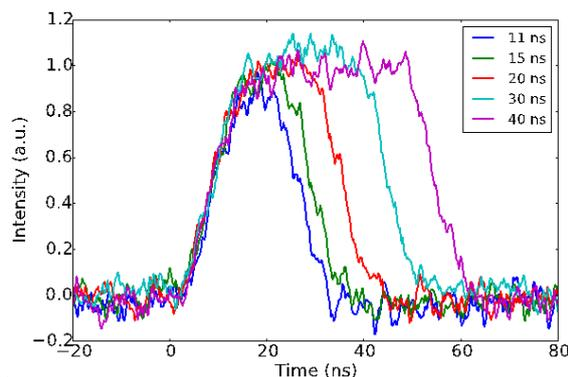
**Figure 6.** Pulses sliced from the CW laser beam by the AOM. The AOM driver was modulated by an SRS DG535 pulse generator; the time markers identifying each trace are the input pulse width from the DG535. The deflected beam is recorded by a Thorlabs DET025AL with 150 ps rise and fall times. The noise on the traces is a results of the low sensitivity of the detector at 1064 nm.
