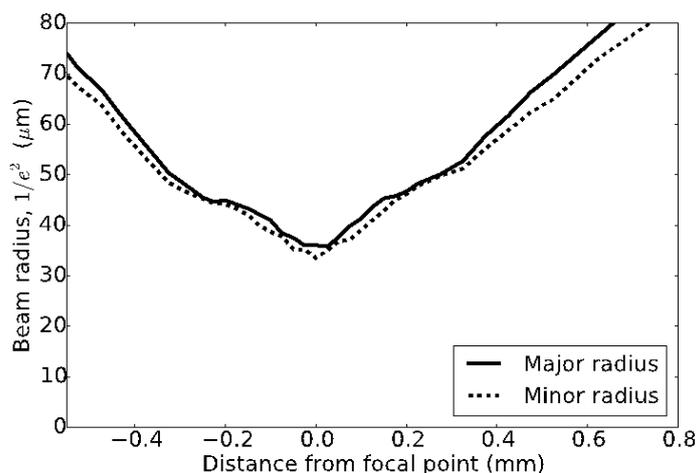
**Figure 4.** The focal spot variation produced by the  $f = +100$  mm lens, with the lens placed approximately 100 cm from the CW laser source.
