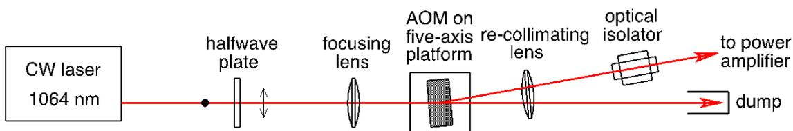
**Figure 1.** A block diagram illustrating the layout of the new master oscillator system. The tilt of the AOM is exaggerated for clarity.
