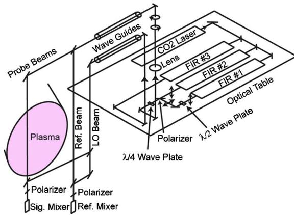
FIG. 1. (Color online) Schematic diagram of the three-wave polarimeter-interferometer for MST. The impact parameters of the 11 probe beams are  $-32$ ,  $-24$ ,  $-17$ ,  $-9$ ,  $-2$ ,  $6$ ,  $13$ ,  $21$ ,  $28$ ,  $36$ , and  $43$  cm, respectively. For clarity, only one probe beam is shown.
