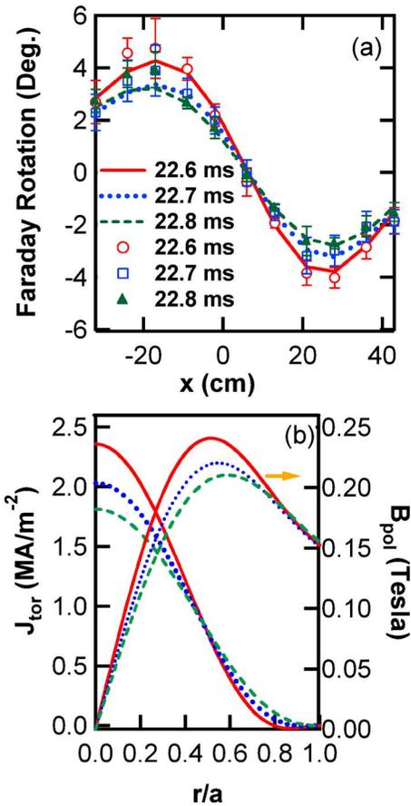
FIG. 4. (Color online) Equilibrium profiles of Faraday rotation (a), current density, and poloidal magnetic field (b) before (22.6 ms), during (22.7 ms), and after (22.8 ms) a single sawtooth crash event. Symbols represent the measurement points and curves are a best fit.
