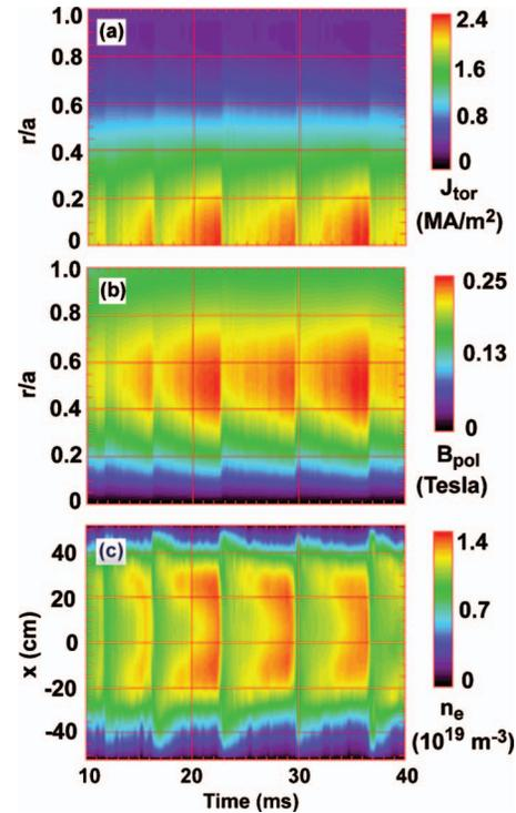
FIG. 5. (Color) Contour plots of (a) toroidal current, (b) poloidal magnetic field, and (c) electron density profile evolution in MST. At sawtooth crashes,  $J_{\text{tor}}$  on the axis collapses from  $\sim 2.5$  to about 1.8 MA/m<sup>2</sup>.
