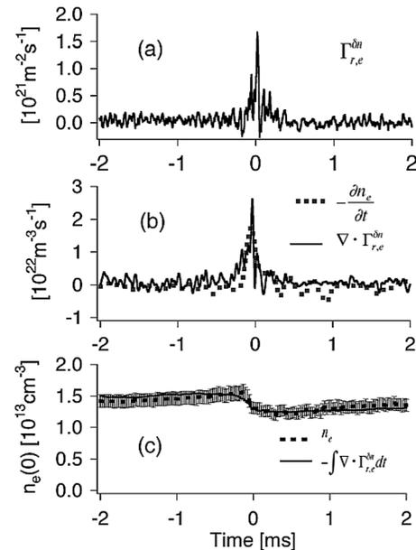
FIG. 3. (a) Electron particle flux, and (b) divergence of density fluctuation-induced electron flux vs time at  $r/a = 0.11$  (solid line). Dashed line denotes time derivative of equilibrium density. (c) Time integrated flux divergence (solid line) and electron density (dashed line). The density at  $t = -0.475$  ms is taken as an integral constant. All results shown are for a sawtooth cycle (crash occurs at  $t = 0$ ).
