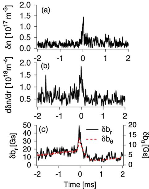
FIG. 2 (color online). (a) Density fluctuation, (b) density fluctuation gradient, and (c) radial magnetic field fluctuation (left vertical axis) during sawtooth cycle (crash at  $t = 0$  at  $r/a = 0.11$ ). Dashed line in (c) shows poloidal magnetic field fluctuation amplitude (right vertical axis) as measured at wall.
