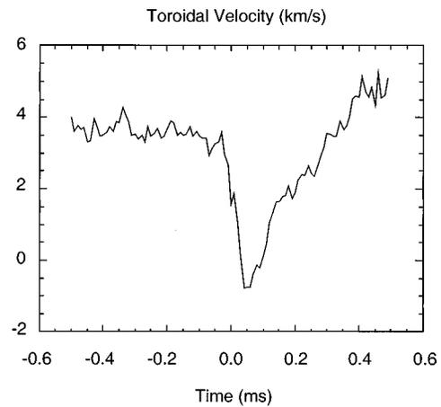
FIG. 2. Plasma braking during a sawtooth event. The plasma toroidal velocity was measured at an insertion point (as determined by the crossing of the view lines) of 5 cm from the wall. The rotation velocity was determined by Doppler shift of the He II 468.6 nm.
