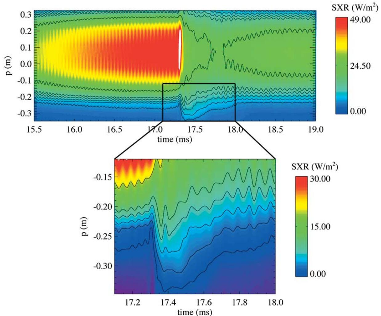
Fig. 1. (a) Contour plot of the SXR brightness measured as a function of the impact parameter  $p$  and of the time during a PPCD discharge in the MST experiment. (b) Zoom of the above plot, which shows in greater detail the propagation of a heat pulse from the hot plasma core toward the edge. Color bar indicates the values of the SXR brightness in the two cases.
