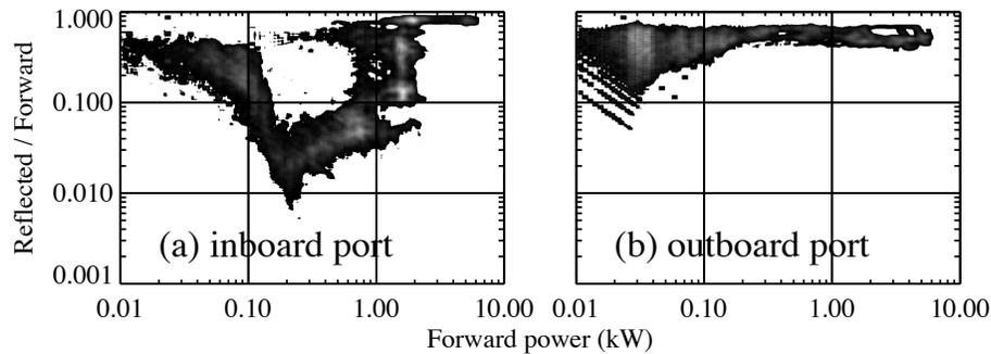
**FIGURE 2.** The antenna behavior in the presence of RFP plasma over many shots is displayed in a contour plot. When fed from the inboard port (a) the reflected power decreases until it reaches a level of < 10% and at a power level of ~2-3 kW it increases abruptly to nearly fully reflecting. When fed from the outboard port (b), the antenna is always nearly fully reflecting.
