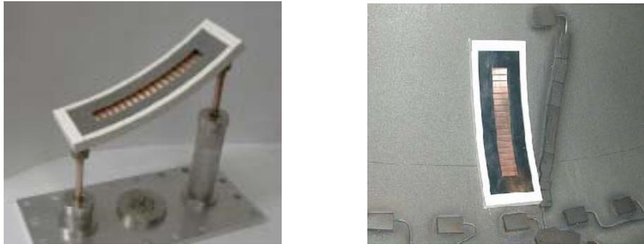
**FIGURE 1.** Pictures of the fully assembled antenna. The picture on the left shows the antenna on the bench with the flange and vacuum / power feed-thru. The longer of the two feed-thrus is located furthest to the inboard side of MST. The picture on the right shows the antenna installed in MST in October 1999 (the plasma facing components and rods are molybdenum; edge limiter is boron nitride).
