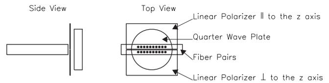
FIG. 3. Drawing of the configuration of the quarter wave plate, filter, and fiber bundles. Each of the fiber pairs views through a linear polarizer and then through the quarter wave plate.
