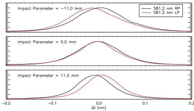
FIG. 4. (Color online) Normalized raw spectral data from three chords through the pinch plasma shows the shift of the right polarization (RP) and left polarization (LP) from the C IV doublet. The shift is plotted relative to the static wavelengths for each line of the doublet. The direction and magnitude of the shifts of the RP and LP are consistent with a Z-pinch magnetic field centered at the geometric center.
