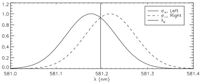
FIG. 1. The spectral intensity measured with a quarter wave plate and linear polarizer show the shift due to Zeeman splitting. The peak of the intensity shift between the right hand circularly polarized (dashed) and the left hand circularly polarized (solid) view is proportional to the magnetic field. The unshifted wavelength is shown for reference.
