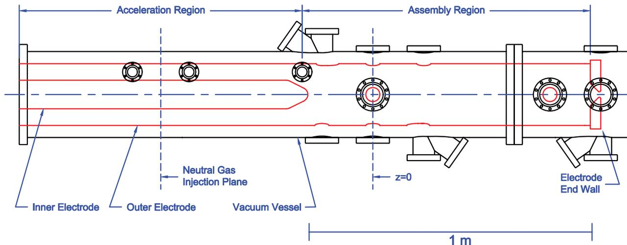
FIG. 2. (Color online) Drawing of the ZaP experimental apparatus is shown. The drawing identifies the key features — the acceleration region, assembly region, and the  $z = 0$  plane. Zeeman splitting measurements are made through the bottom port at  $z = 0$ . A 1 m scale is included for reference.
