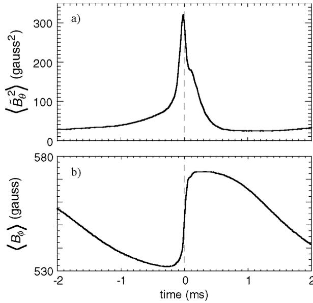
**Figure 2.** Variation in (a) the magnetic field fluctuation amplitude and (b) the average toroidal magnetic field over a sawtooth cycle in MST from an ensemble average of several hundred sawtooth events. The time of the maximum increase of the toroidal magnetic field defines  $t = 0$ .
