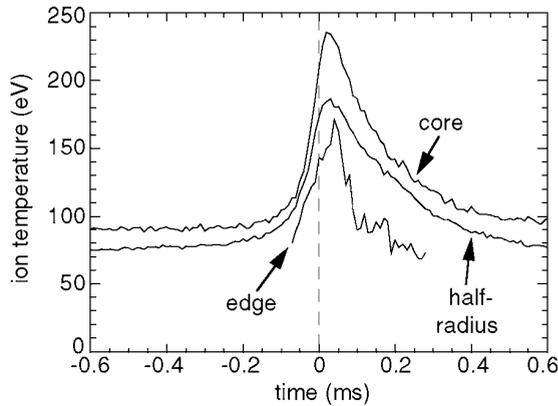
**Figure 5.** Measurements from core, half-radius and edge viewing chords confirm that ion heating occurs simultaneously across the minor radius during a sawtooth crash.
