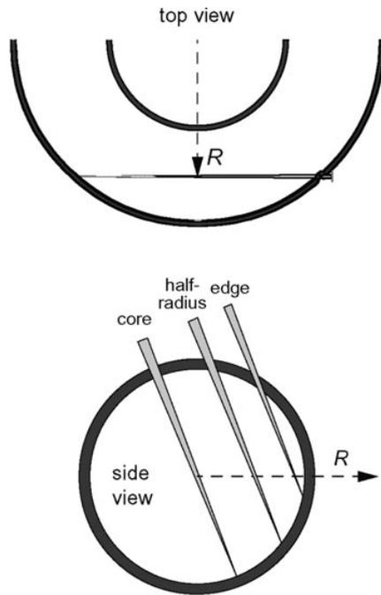
**Figure 1.** Viewing chords for Doppler spectroscopy on MST. The top view shows the toroidal viewing chord which passes through the central core of the plasma. The side view (below) is illustrative of the radial viewing chord ( $r/a = 0$ ) and half-radius and edge chords.
