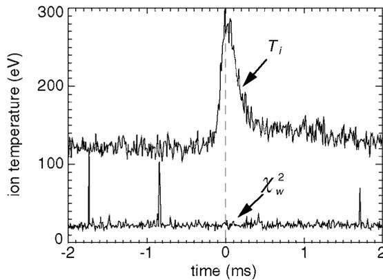
**Figure 4.** The weighted  $\chi_w^2$  of the Gaussian fits for the toroidal viewing chord over a sawtooth cycle, illustrating the lack of non-Maxwellian distortion of the ion velocity distribution function, even during strong heating. The radial viewing chord shows similar behaviour. This data is from a set of 300 kA MST discharges, thus  $T_i$  is higher than in figure 3.
