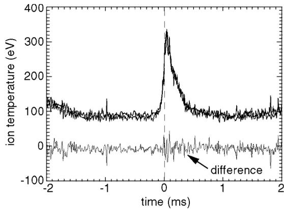
**Figure 6.** Perpendicular  $T_{\perp}$  from two toroidally separated viewing chords, and the difference between them, further illustrating the spatial symmetry of ion heating.
