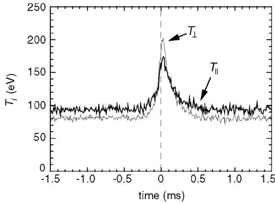
**Figure 3.** Parallel and perpendicular impurity ion temperatures over a sawtooth cycle. The ions are strongly heated around  $t = 0$  when the sawtooth crash occurs and the MHD activity is largest.
