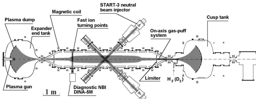
FIG. 1. The GDT layout.
