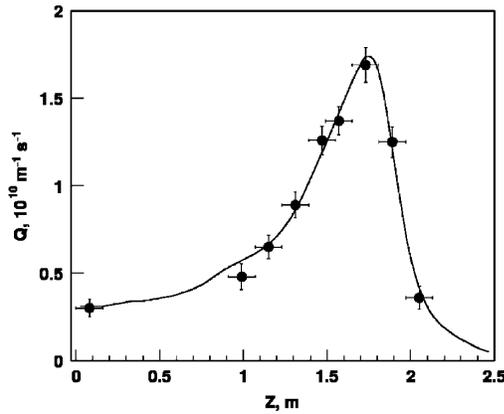
FIG. 3. Axial profile of DD reaction yield as measured from the midplane ( $z = 0$ ).
