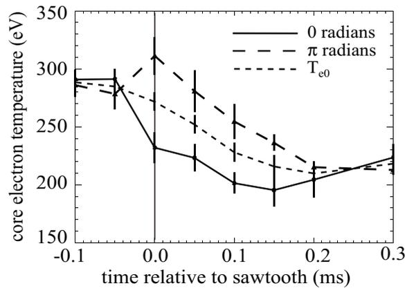
**Figure 5.** Comparison of core electron temperature at  $\Delta_{TS} = 0$  and  $\Delta_{TS} = \pi$  with the equilibrium electron temperature,  $T_{e0}$ . Errors are propagated through the calculations using the widths of the final PDFs.
