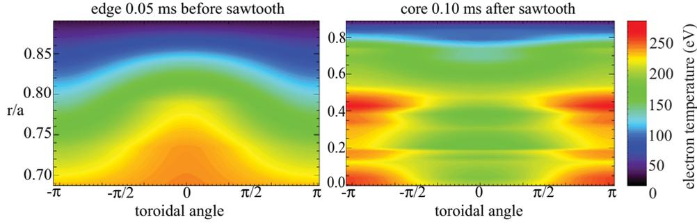
**Figure 3.** (Left) contour plot of the electron temperature at the edge of MST prior to the sawtooth. Heat is confined at  $\Delta_{TS} = 0$  compared with  $\Delta_{TS} = \pi$ . (Right) contour plot of the electron temperature variation due to (0,1) correlated fluctuations after the sawtooth, from core to edge. Note that the ordinate range of the plots differs.
