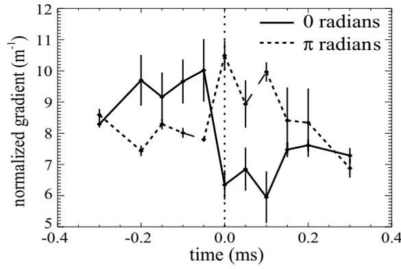
**Figure 4.** Normalized edge electron temperature gradient at the O-point (0 radians) and the X-point ( $\pi$  radians) of the magnetic island through the sawtooth crash.  $t = 0$  is denoted by the vertical line. Errors are propagated through the calculations using the widths of the final PDFs.
