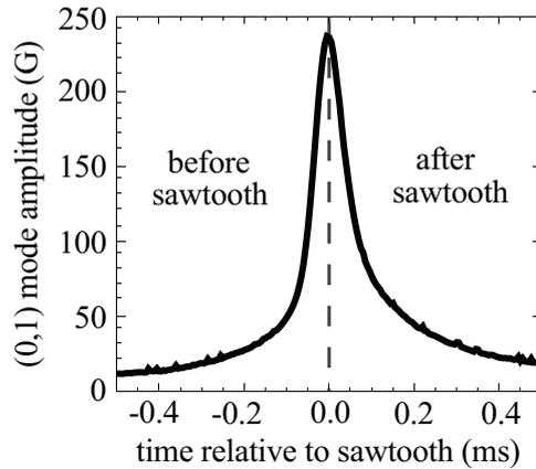
**Figure 1.** Ensemble-averaged (0, 1) mode amplitude through the sawtooth crash, measured at the wall.  $t = 0$  is plotted as a vertical dashed line.
