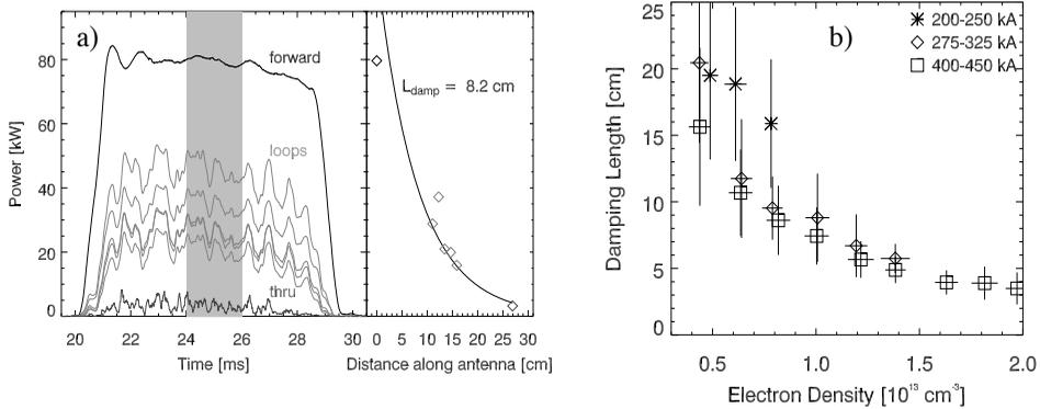
**FIGURE 1.** (a) Calculation of damping length of RF power flowing down the antenna. (b) Damping Length vs. Density for several different plasma currents.
