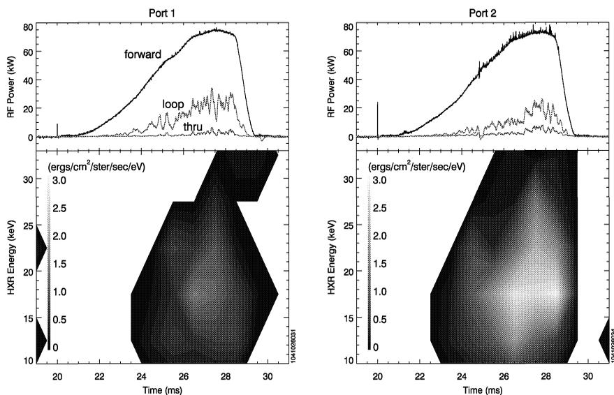
**FIGURE 3.** Plot of hard x-ray flux vs RF power for both feed directions.
