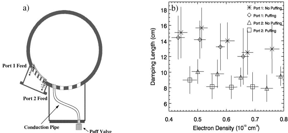
**FIGURE 2.** (a) Diagram of localized puffing apparatus near the lower hybrid antenna. (b) Damping length vs. line-averaged density for local puffing on ports 1 and 2.
