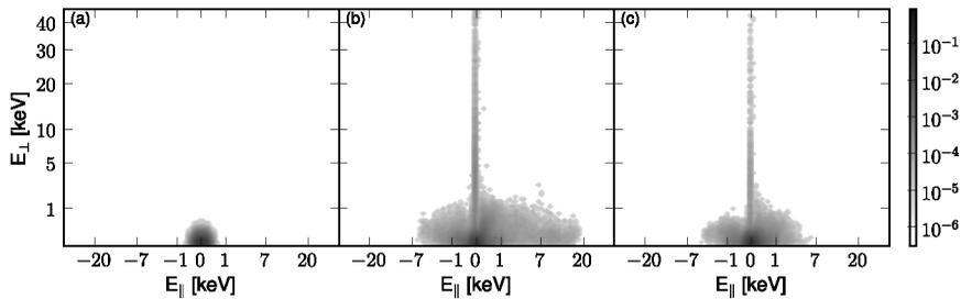
**Figure 4.** Results from Monte Carlo calculation. (a) Initial 40 eV distribution. (b) Final distribution for 85 kW input power and guide field pitch angle  $8^\circ$  relative to the antenna axis. (c) Same as (b) but with a power damping length of 5 cm on the antenna.
