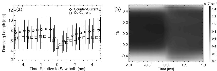
**Figure 1.** (a) The antenna damping length relative to the sawtooth cycle in 400 kA plasmas for both antenna phasings. (b) The density profile at the midplane for these plasmas. Zero milliseconds corresponds to the sawtooth crash.
