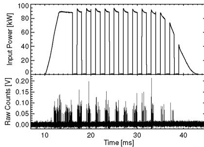
**Figure 3.** The rf power modulated at 500 Hz and the HXR response.
