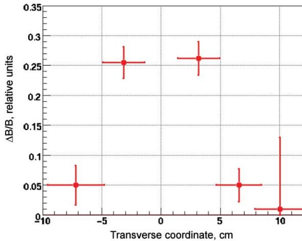
FIG. 3. (Color online) Radial profile of the diamagnetic field reduction  $\Delta B/B$  in the fast ion turning point.
