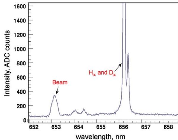
FIG. 2. (Color online) Sample spectrum acquired in hot-plasma GDT shot. Magnetic field in plasma calculated by the beam emission spectrum:  $|B_z| = 0.437$  T.
