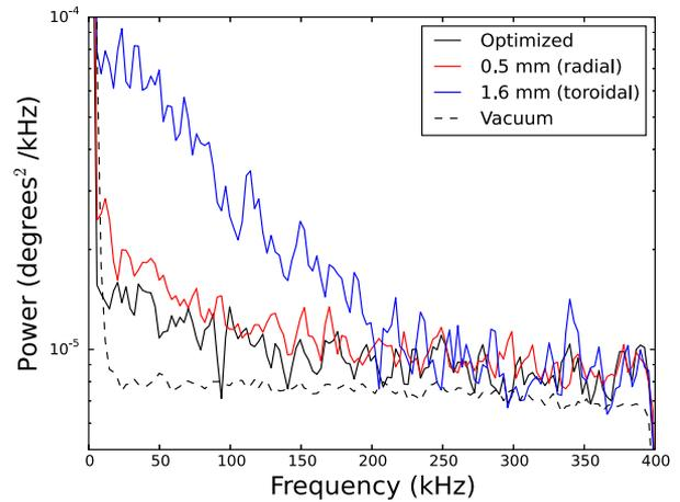
FIG. 2. Power spectra for the chord closest to the magnetic axis ( $R - R_0 = 6$  cm) with both probe beams in the same polarization state. Displacements of 1.6 mm (toroidal) and 0.5 mm (radial) are compared to the optimized spectrum ( $\leq 0.1$  mm).
