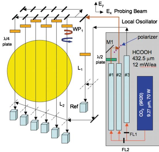
FIG. 1. Schematic of three-wave FIR polarimeter-interferometer. Two probe beams with orthogonal polarization pass through the plasma for polarimeter operation, while a third beam serves as the local oscillator for interferometer operation. Only six chords are shown for simplicity.
