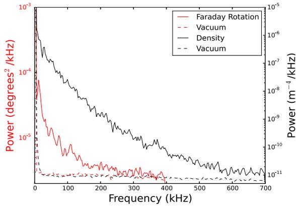
FIG. 3. Power spectral density for Faraday rotation and density between sawtooth events for a central chord near the magnetic axis ( $R - R_0 = -2$  cm).
