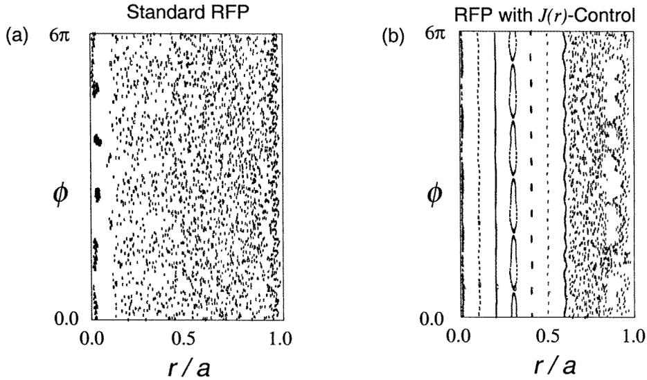
**Figure 7.** MHD prediction for the magnetic field line puncture plot in the radial-toroidal plane (a) without auxiliary current drive and (b) with auxiliary current drive.
