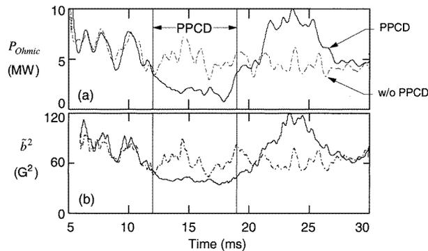
**Figure 8.** Magnetic fluctuations and ohmic input power against time, with and without pulsed poloidal current drive (PPCD) in MST.
