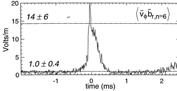
**Figure 4.** One component of the MHD dynamo ( $\langle \delta v_\phi \delta B_r \rangle$ ), contributed from the toroidal mode number  $n = 6$ , as a function of time through a sawtooth cycle. Velocity fluctuations were measured by Doppler spectroscopy in the MST core and magnetic fluctuations by an edge coil array.
