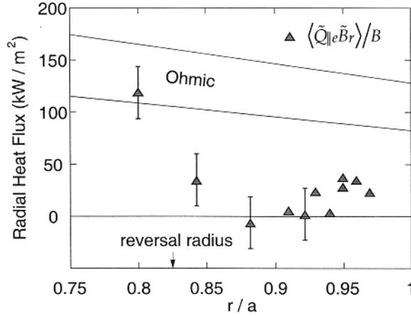
**Figure 5.** The radial electron energy flux driven by magnetic fluctuations against radius. The shaded region is the estimated total energy flux.
