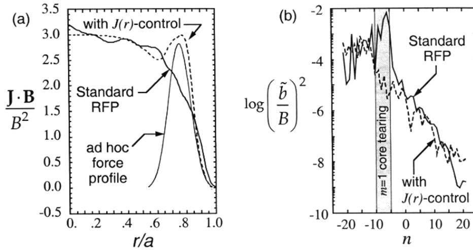
**Figure 6.** Prediction of nonlinear, resistive MHD computations for (a) the current density profile against radius in the outer region and (b) the toroidal mode number spectrum of magnetic fluctuations, both with and without auxiliary current drive in the outer region.
