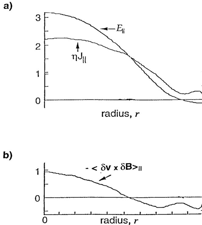
**Figure 2.** The radial profile of each term in the parallel mean-field Ohm's law, equation (1), showing (a) the mean electric field and current density terms and (b) the fluctuation-induced dynamo term, computed from nonlinear, resistive MHD equations.
