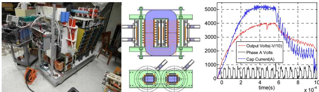
**FIGURE 3.** (A) Power supply, (B) Resonant transformer design, and (C) Voltage waveform during arc (red:voltage, blue:current, black: phase A primary voltage)
