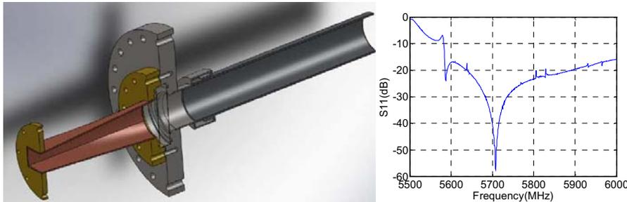
**FIGURE 2.** (A) Pillbox window design showing tapered rectangular to circular transition, quartz window, vacuum flange, and molybdenum antenna and (B) Pillbox window S11 parameters showing sharp resonance slightly offset from at 5.55GHz.
