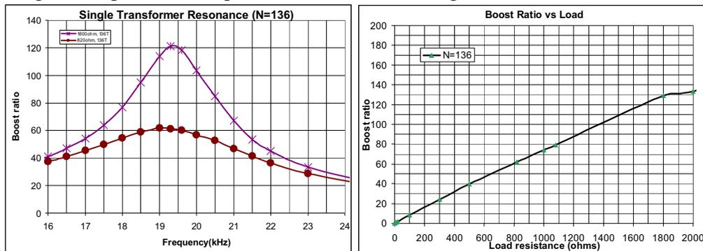
**FIGURE 4.** (A) Transformer boost ratio vs frequency, and (B) Boost ratio vs Load.
