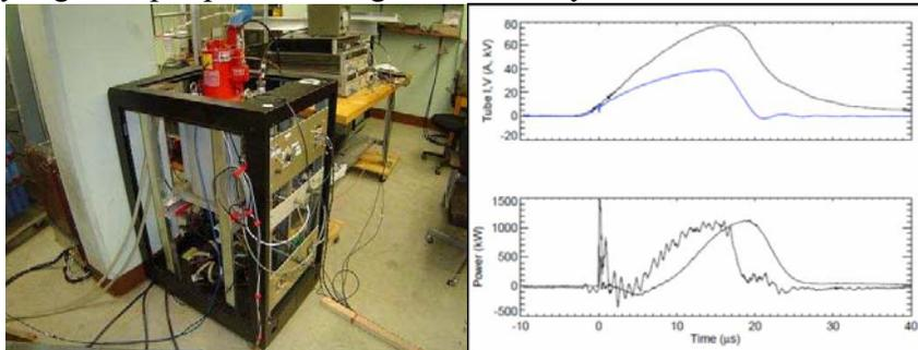
**FIGURE 1.** (A) Klystron tube and (B) Measured short pulse output (Top: black-tube voltage, blue-tube current, Bottom: tube power measurements through two different detectors. Note: the shift in time between the plots is due to phase lag of an amplifier).
