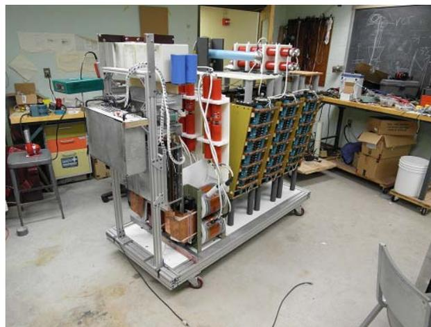
Figure 1. Three phase resonant power supply.
