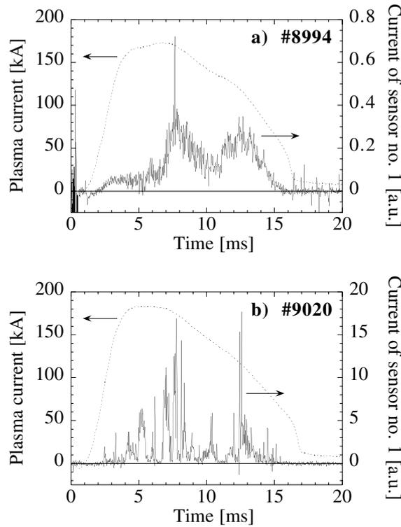
**Figure 3.** Main plasma current and typical waveforms of pyrosensor current: (a) slit located at  $r/a = 1$ ; (b) slit inserted at  $r/a = 0.88$ .
