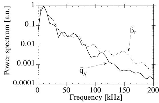
**Figure 6.** Power spectra of parallel energy flux,  $\tilde{q}_{\parallel}$ , and of radial magnetic field,  $\tilde{b}_r$ .
