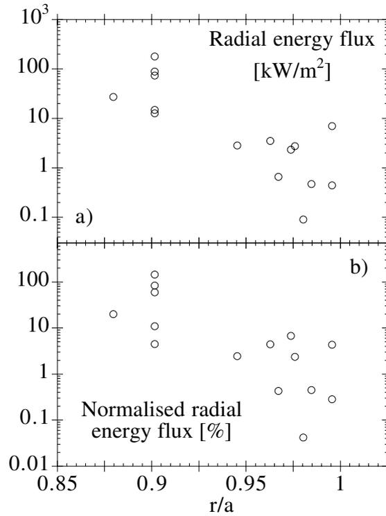
**Figure 7.** Radial energy flux (upper frame) and radial energy flux normalized to global energy flux (lower frame) as a function of the radial position of the detector.
