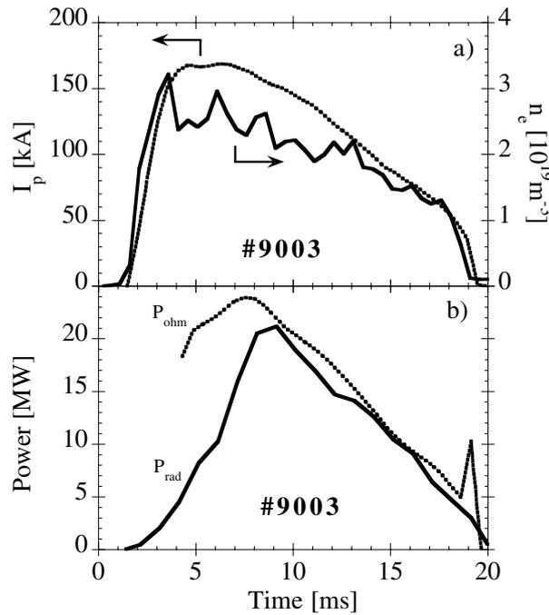
**Figure 2.** Main plasma parameters: (a) toroidal current and electron density; (b) ohmic and radiated power.
