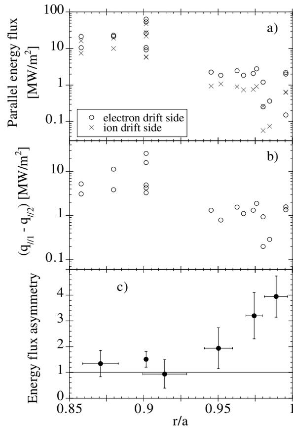
**Figure 4.** Parallel energy fluxes (a), net parallel energy flux (b) and energy flux asymmetry (c) as a function of the probe radial position.
