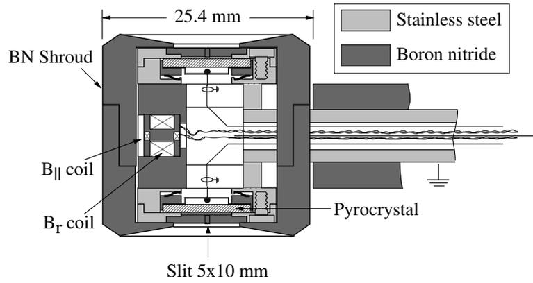
Figure 1. Schematic view of pyrobolometer equipment.
