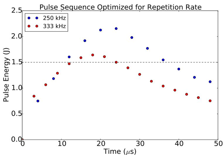
**Figure 4.** By using the Nd:glass stages for energy storage and increasing their pumping time before pulsing, the pulse sequence can be optimized for fastest repetition rate. The pulse energies plotted here are the current best for 250 and 333 kHz.
