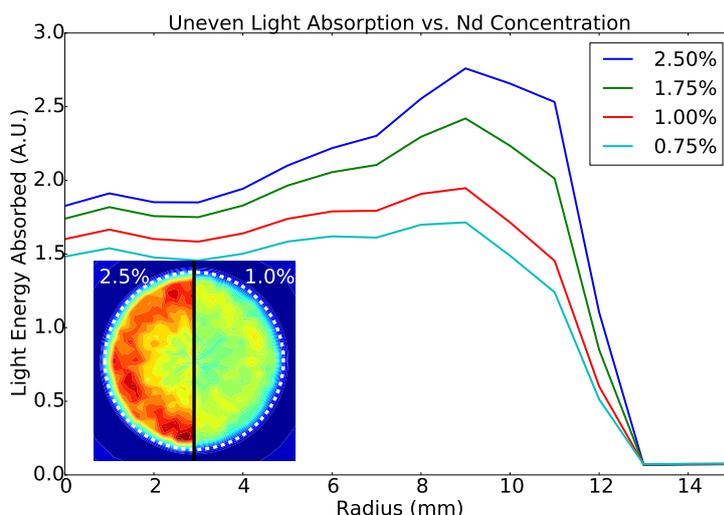
**Figure 2.** The above plot shows the radial profile of light absorption with a Nd:glass rod with difference concentrations of Nd ( $\text{Nd}_2\text{O}_3$  by weight). 2D contours of the light absorption for two concentrations are shown in the insert (warm colors for more absorption). The white dashed circle marks the edge of the rod. The original 2.5% rods were replaced with 1% rods.
