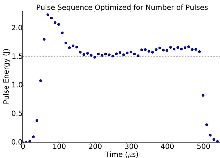
**Figure 3.** This sequence of pulse energies is the largest number of pulses achieved so far in a single burst: 44 pulses at 100 kHz.
