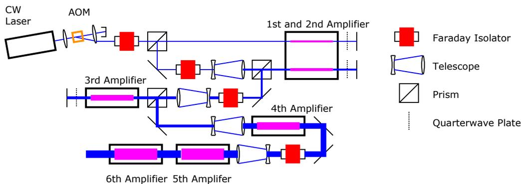
**Figure 1.** Above is a diagram of current components of the high-repetition-rate laser with most mirrors removed to simplify the diagram.
