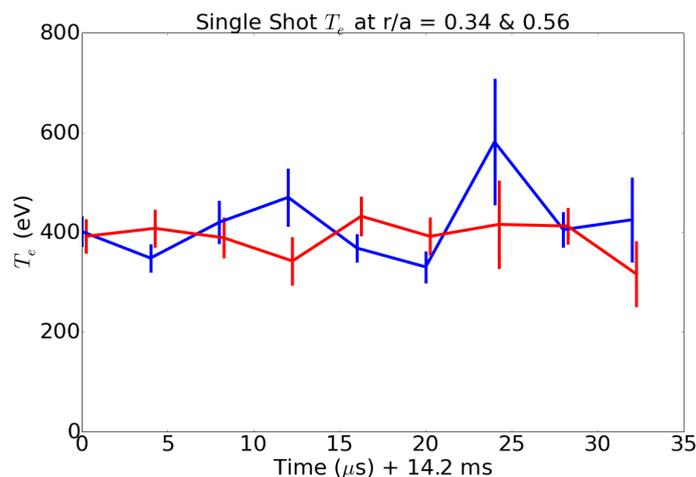
**Figure 5.** The temperature data from two chords is plotted here to show average to smaller than average error bars for MST TS measurements (10-20%) at 250 kHz. This data was taken when the laser only had five amplifiers installed.
