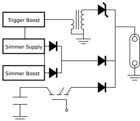
**Figure 4.** This diagram shows a simplified schematic of the circuits driving the flashlamps in both of MST's Thomson scattering lasers. The capacitor at the bottom is the main capacitor to drive the flashlamps during pulsing, switched by the IGBT. The simmer sources and main IGBT are protected by a 20 kV of diode stacks, while the output of the trigger transformer has 2 kV of transient voltage suppressor diodes.
