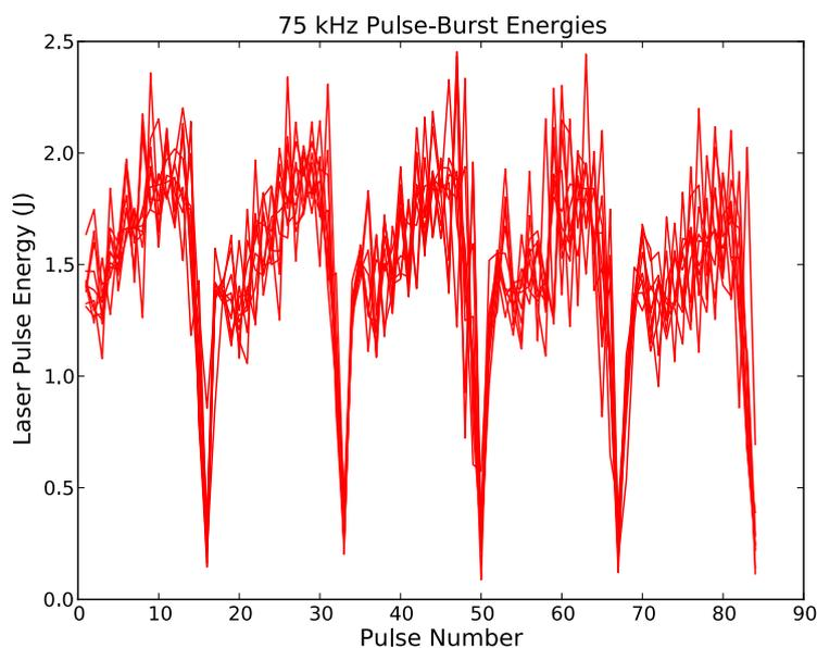
**Figure 3.** Laser pulse energies for operating in pulse burst mode, with 5 bursts of 15 pulses. The pulses within a burst are at a rate of 75 kHz, while the bursts are at a rate of 1 kHz. An extra pulse after the flashlamps are exhausted, and hence at 0 J, was left in each burst to mark the points between bursts instead of plotting the longer idle time.
