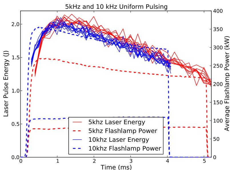
**Figure 2.** Laser pulse energy and flashlamp power are plotted when operating at a uniform pulse repetition rate of 5 kHz and 10 kHz. The larger flashlamp power curve for each frequency is the average of three of the six 8 mm bore flashlamps in the Nd:glass stage, the smaller curves are an average of the seven, 4 mm bore flashlamps in the Nd:YAG stages. 10 shots worth of laser pulse energies are plotted to illustrate pulse to pulse variability.
