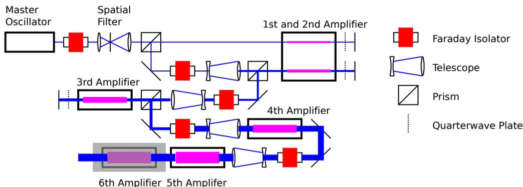
**Figure 1.** This is a simplified diagram of the high repetition laser, showing all optical components except for some mirrors.
