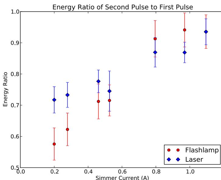
**Figure 6.** This plot shows the ratio of the second pulse energy to the first pulse energy in a sequence of pulses at 500 Hz, versus several different simmer currents. At low currents, there is up to a 40% drop in flashlamp energy and 30% drop in laser pulse energy, but this saturates to about a 10% drop at higher currents.
