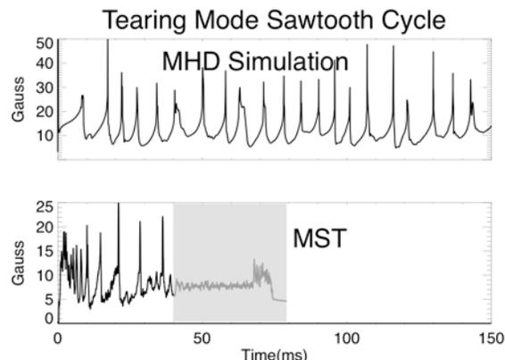
Fig. 7. Sawtooth cycle in MST and MHD computation, representing the opportunity for validation of nonlinear MHD. The shaded region for MST is the ramp-down phase when the drive for tearing instability is reduced.
