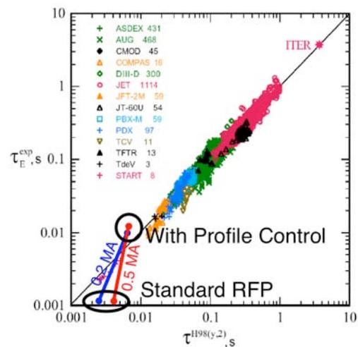
Fig. 6. MST confinement compared to tokamak H-mode empirical scaling. (Reprinted from ITER Physics Guidelines, ITER report N 19 FDR 1 01-07-13 R 0.1.)
