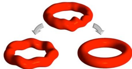
Fig. 5. Two pathways for improved RFP confinement: Quasi-single-helicity self-organization (left) and profile control for tearing stability (right). The plasma distortion is magnified for illustration purposes.
