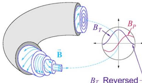
Fig. 2. Schematic of the RFP magnetic configuration. The toroidal and poloidal field components are similar in magnitude, yielding a highly sheared magnetic geometry.
