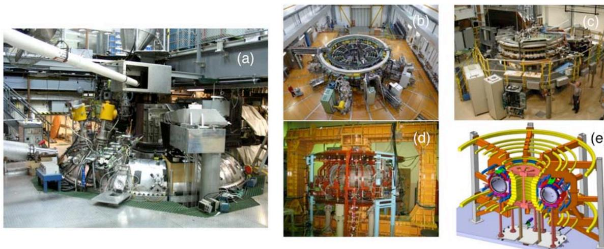
Fig. 3. World's RFP facilities: (a) MST,  $I_p = 0.6$  MA,  $a = 0.5$  m,  $R = 1.5$  m (b) RFX-mod,  $I_p = 2$  MA,  $a = 0.4$  m,  $R = 2$  m, (c) Extrap-T2R,  $I_p = 0.3$  MA,  $a = 0.18$  m,  $R = 1.24$  m, (d) RELAX,  $I_p < 0.1$  MA,  $a = 0.25$  m,  $R = 0.51$  m, (e) KTX,  $I_p = 1$  MA,  $a = 0.4$  m,  $R = 1.4$  m (under construction)
