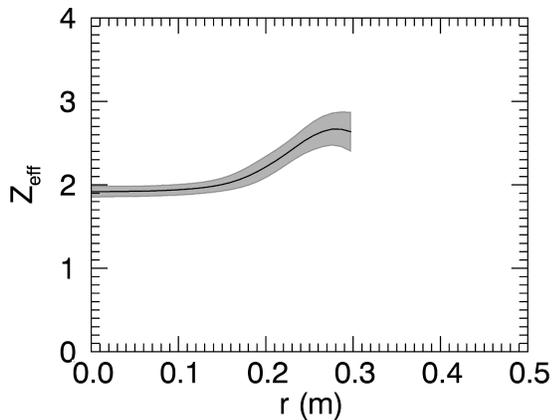
Fig. 1. Most probable radial profile of  $Z_{\text{eff}}$  in the core of MST, produced by integrating data from CHERS and SXR tomography measurements using the techniques of IDA. Lack of SXR data outside of  $r/a = 0.3$  currently constrains the measurement to the core region; it is not an inherent limit of the technique.
