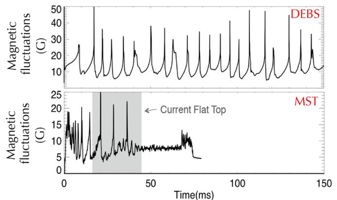
Fig. 1. Temporal evolution of magnetic fluctuations, summed over dominant tearing modes, from DEBS simulation and from an MST plasma. Courtesy of J. Reusch.
