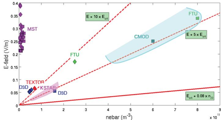
Fig. 2. Onset and suppression thresholds for runaway electrons (IAEA 2014). Courtesy of R. Granetz.
